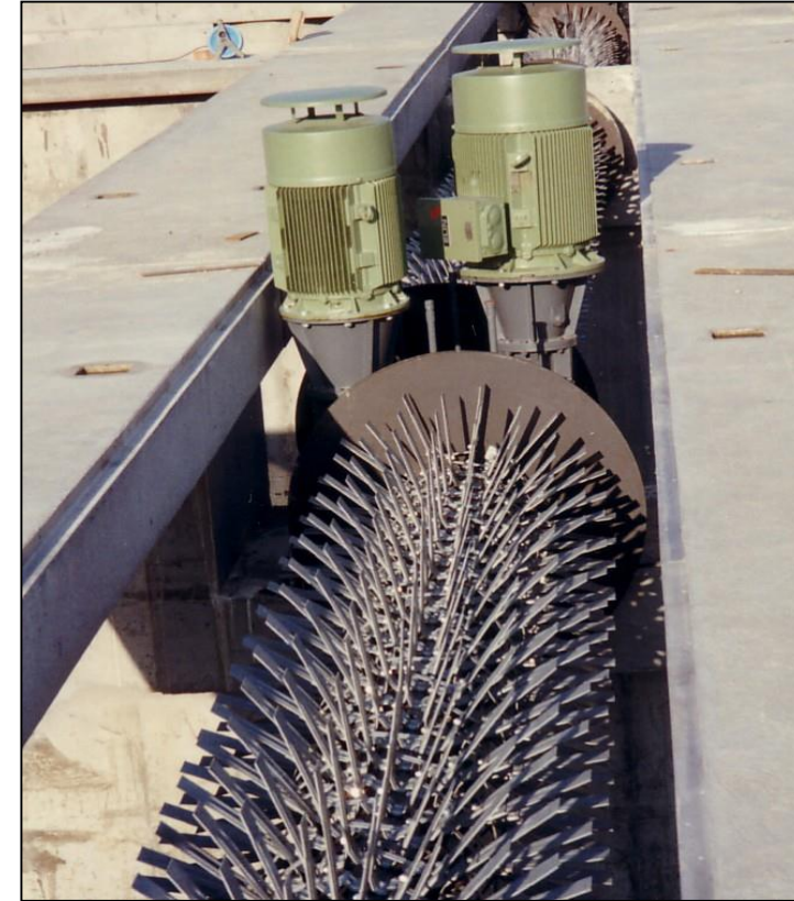
Aeration rotor \varnothing 1.000mm
